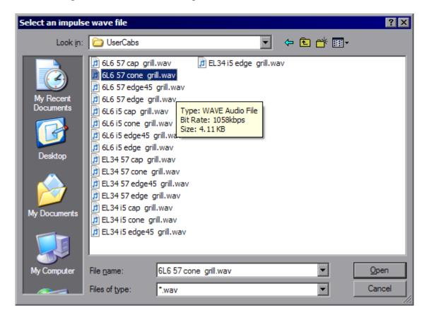
The updater will then load the cabinet to any program so you can instantly hear the effect of the new user. If you selected make cabinet permanent the 1101 will write the cabinet to flash and reboot. Once the unit has rebooted the cabinet will be available.
